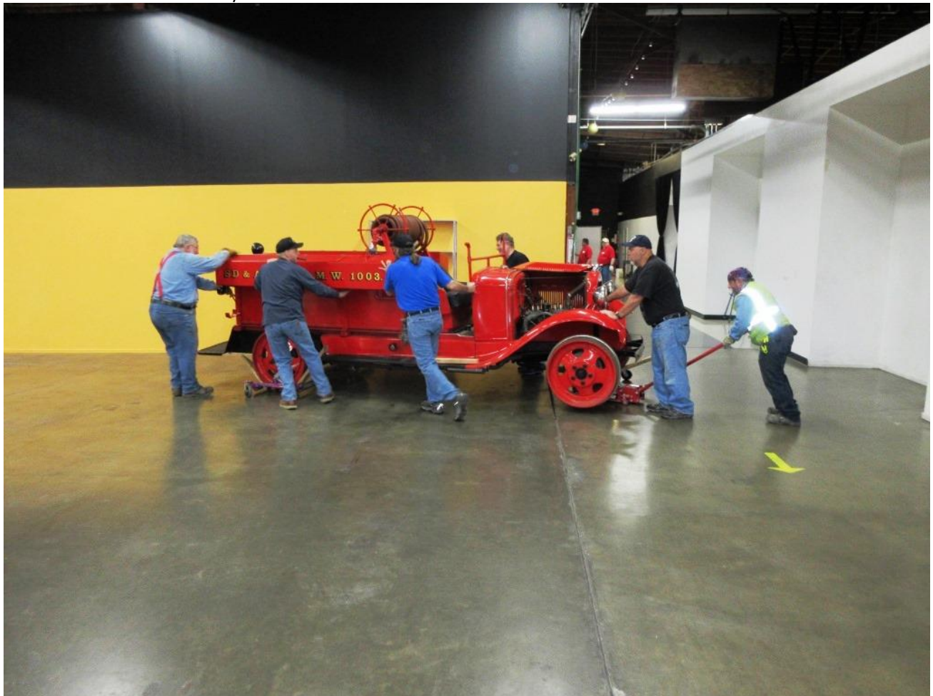
Using a rolling-jack and special wheelie-dealies, the fire-truck is maneuvered into position
