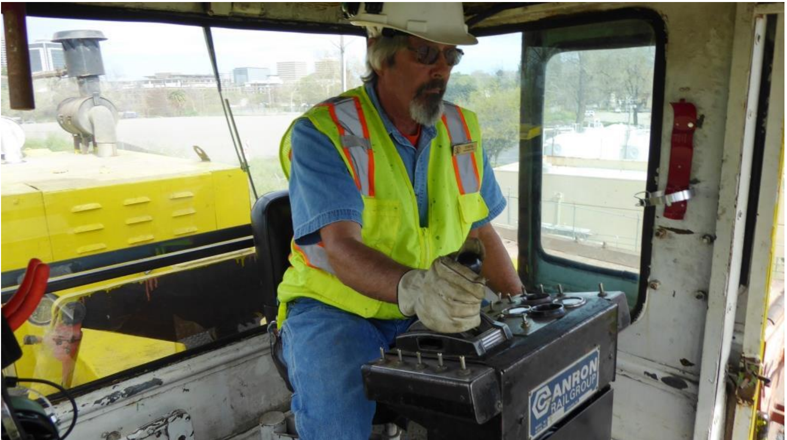
Ed has a firm hand on the controls of the ballast regulator while plowing newly laid rock
